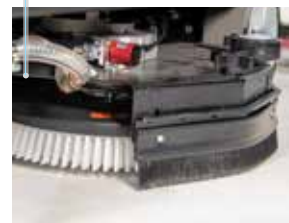
Double Brush Motors Delivers powerful and consistent scrubbing performance
